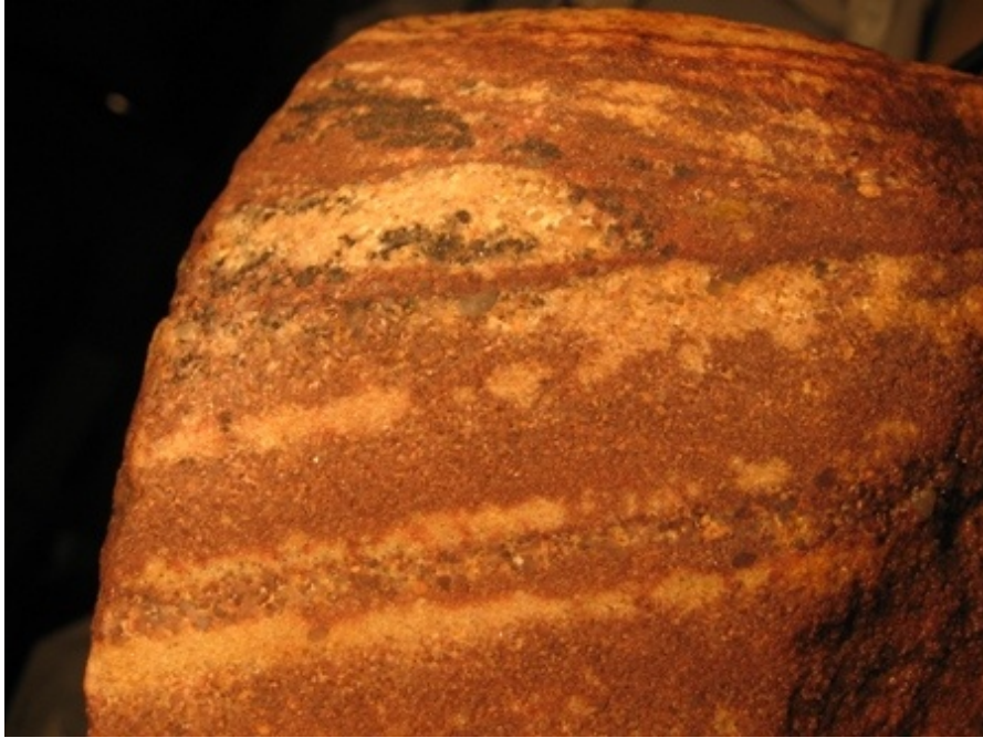
Fig.16 Chip of Riphean sandstone (second sample) The size of the fragment is 10 cm
